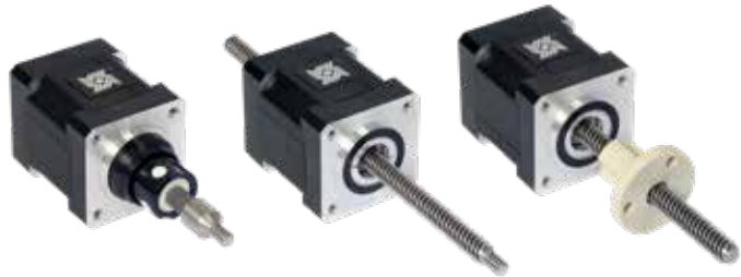
Figure 11. Hybrid Linear Actuators Size 17 Series. (43mm square) Captive, Non-captive and External Linear, available in 1.8 and 0.9 rotational degrees per step.
