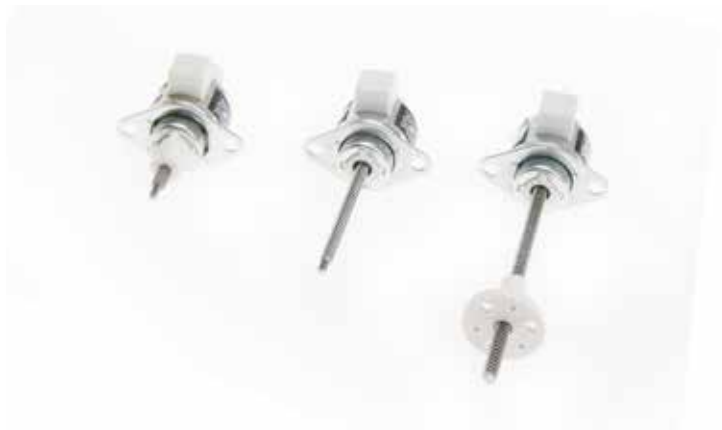
Figure 12. Can-Stack Linear Actuators. 19000 Series (20 mm) Captive, Non-captive and External Linear, available in 15 and 7.5 rotational degrees per step.
